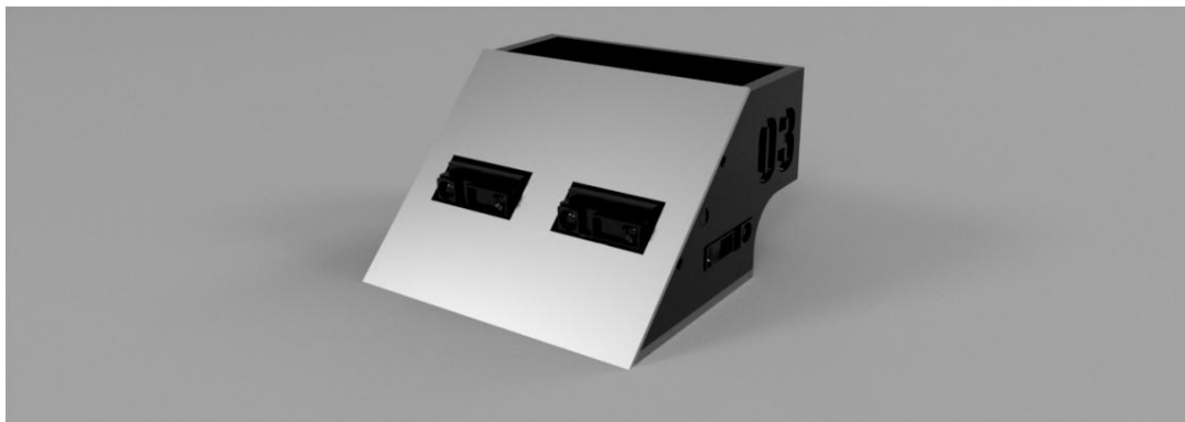
NEMO 03 in the projection, visible "plow" with rectangular openings for motion sensors, which were placed inside the robot.
