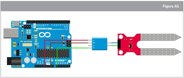
$\uparrow$  The configuration for a moisture sensor with an external controller board.
